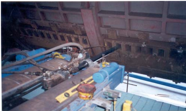
Single Drill Head mounted on Gase Tuyere Puncher
